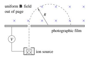
(The little  $\times$ 's represent the magnetic field coming out of the page.) The whole device is enclosed in a vacuum system.
