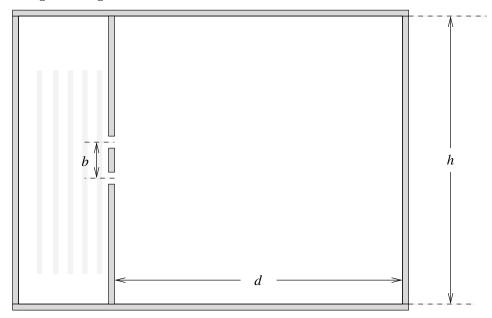
The dimensions are: b = 1.875 in, d = h = 15 in. In the following, ignore any reflections of waves off the sides of the wave tank.
