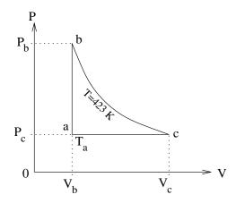
We are given  $T_a = 273 \,\mathrm{K}$ ,  $P_c = 1 \,\mathrm{atm}$ ,  $T = 423 \,\mathrm{K}$ , and  $n = 1 \,\mathrm{mol}$ . Using the ideal gas law,  $V_b P_c = nRT_a$ . Since the curve b-c is isothermal, the ideal gas law tells us  $P_b V_b = P_c V_c = nRT$ . To find efficiency, the work done and heat transferred must be calculated for each process.
